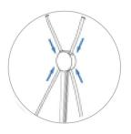
Insert top and bottom graphic arm poles into holes on support pole
